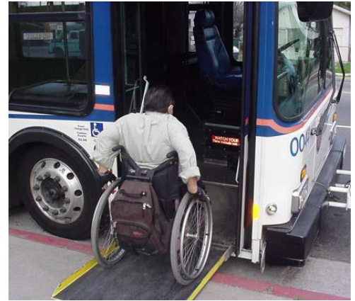
Figure 4 A.D.A. Loading Ramp
